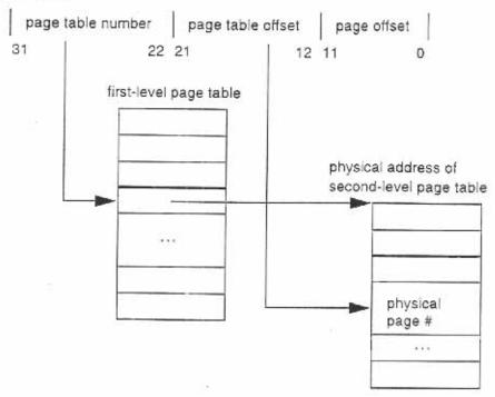
For the peer instruction question, we assumed that the length of a virtual address was 32 bits. List three different ways of accommodating a <u>33-bit</u> virtual address in this address translation system while retaining the two-level table structure and <u>32-bit</u> physical address length. For each method you list, describe its specific effect on page sizes and the page tables.
