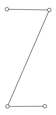
13. Consider this diagram showing a four-joint arm in 2D where each joint is a simple pin joint and the base is fixed in space.
