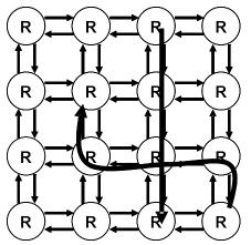
Assume that each router or link has a very small amount of buffer space and that each message can be arbitrarily long. Show a simple situation (with a drawing) in which messages are deadlocked and can make no further progress. Explain how each of the four conditions of deadlock are satisfied by your example. *Hint: Links are the limited resources in this example*.
