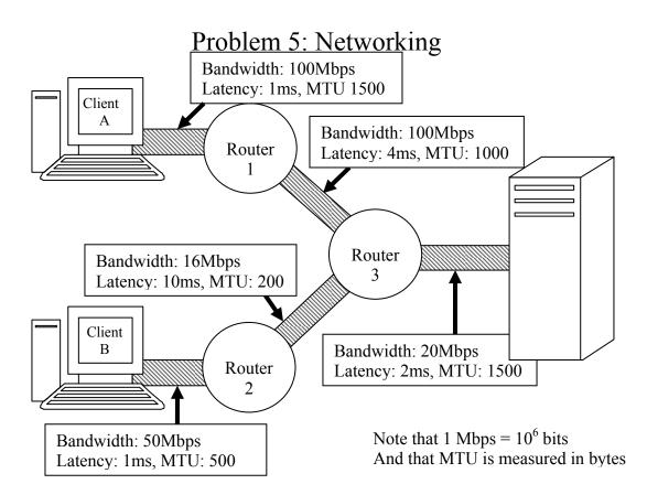
The above figure illustrates a network in which two clients (Client A and Client B) route packets through the network to the server and to each other. Each link is characterized by its Bandwidth, one-way Latency, and Maximum Transfer Unit (MTU) in *bytes*. All links are full-duplex (can handle traffic in both directions at full bandwidth).
