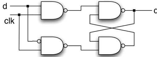
If possible, modify the circuit to achieve the following functions by adding bubbles (inversions) and extra gate inputs (no extra gates or transistors are allowed). If the desired function is not possible, indicate it by writing “not possible”.
