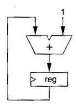
For the circuit shown, assume that the register setup time requirement is 1 ns and the clk to Q delay for the register is 1ns. What is the maximum delay possible through the adder and still guarantee correct operation at 100MHZ?
