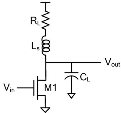
What is the total voltage noise variance  $v_{on}^2$  at the output of the amplifier shown above? You should provide your final answer in terms of  $k$ ,  $T$ ,  $\gamma$ ,  $R_L$ ,  $L_s$ ,  $C_L$ , and  $A_{v0} = g_m R_L$ .
