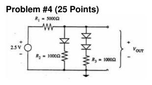
Find  $V_{out}$  in the above circuit. The diodes are to be represented by the large-signal diode model (including the 0.7 V drop across a forward-biased diode.) **Make sure your answer is reasonable and consistent.** Explain your reasoning.
