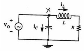
In the above circuit,  $V_0 = 10$  V (real, C = 10^-8 F, L = 2X10^-4 H, R = 100 ohms, omega = 10^6 radians/sec.
