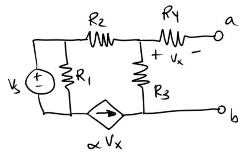
Provide the Thevenin equivalent resistance,  $R_{th}$ , of the circuit above across terminals a,b. Provide a numerical answer with units.
