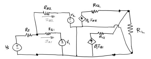
a) Is it possible to set  $\beta 1$  such that  $R_L$  delivers 1 W to the rest of the circuit? If so, what is the value of  $\beta 1$  that will accomplish this?
