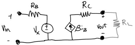
What value should R<sub>C</sub> have such that maximum power is transferred to R<sub>L</sub>? (2 points)
