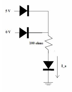
0V diode is off, 5V diode and I\_a diode are on.
