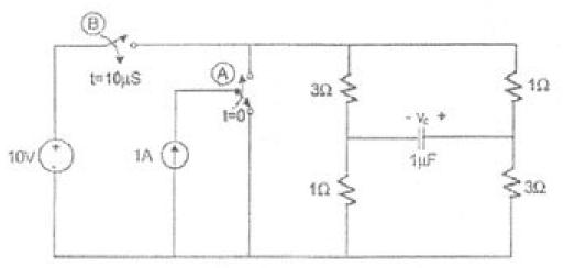
The circuit shown here is at equilibrium with  $v_c = 0$  at t = 0. At t = 0, switch A is moved as shown in the diagram. Then at time  $t = 10 \ \mu\text{S}$ , switch B is closed.
