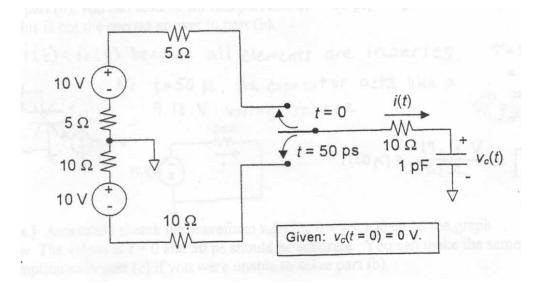
(a) [4 pts] What is the value of the current i (t =  $0^+$ ) in Amperes? The switch moves up at t = 0 and down at t = 50 ps. (note that 1 ps =  $10^{-12}$  s).
