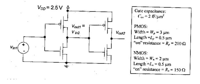
(a) [4pts.] This inverter pair als been "at rest" for some time with its input "high." The wave for for  $v_{in1}(t)$  is sketched below. Draw teh switch-model circuit for finding the output voltage  $v_{out1}(t)$  of inverter 1 for t > 0. Provide some numerical values for the circuit elements. You can neglect the drain-bulk capacitances and any wire capacitance.
