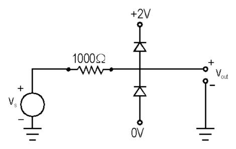
In the above circuit, the diodes are to be represented by the large signal diode model, (the one that looks like this:)
