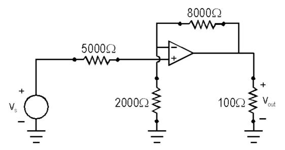
The voltage v<sub>s</sub>(t) is an endless sinusoid with frequency 1MHz and amplitude 2V, as shown here:
