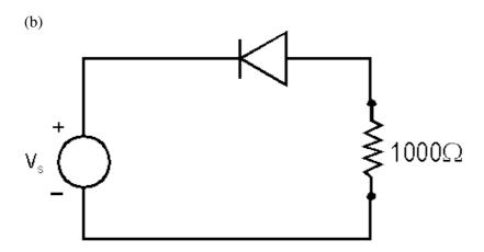
$v_s$  and the diode are the same as in part (a). Find the time-averaged power dissipated in the diode, averaged over the 4-second period.
