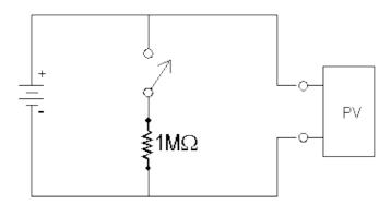
When the switch is open (not connected) the physical voltmeter reads 8 volts. When the switch is closed (connected) the physical voltmeter reads 6 volts. Rind R<sub>B</sub> and V<sub>B</sub>.
