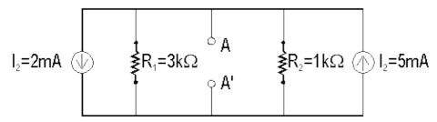
A two-terminal subcircuit is shown with terminals A and A'. Find its Th&#233 venin equivalent, making your method clear. (Label the terminals AA' in your equivalent circuit)
