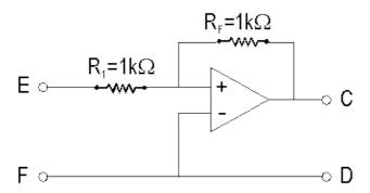
In the above circuit the op-amp has an abnormally low voltage amplification; in fact, A=5. Its input resistance  $R_{i=1}M^{\Omega}$  and  $R_{o=0}$ . Output terminals C, D, are open-circuited.
