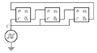
In the circuit above, the flip-flops are positive-triggered D flip-flops. The truth table is repeated for your convenience.
