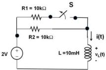
(a) (3 points) For time t <0, the switch S is closed and the circuit is at steady state. What is the value of current i?
