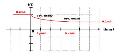
$$\begin{aligned} v_L(t) &= L \bullet di/dt \\ &= - (10 \text{mH} \bullet 2 \bullet 10^{-4} \text{ Amp/} 10^{-6} \text{ sec }) \bullet \text{exp(-t/} 1 \mu \text{sec)} \\ &= -2 V \bullet \text{ exp(-t/} 1 \mu \text{sec)} \end{aligned}$$
