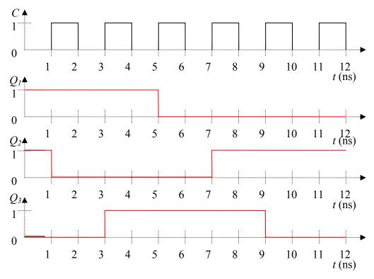
b) What are the periods of the clock (*T*) and *Q* signals ( $T_n$ )? Give correct units. (3 pts) T = 2 ns,  $T_n = 12$  ns
