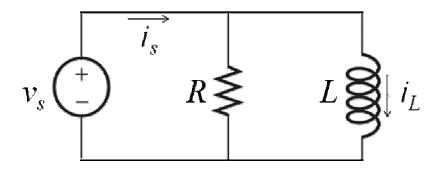
$R = 3 \Omega$ , L = 1 H,  $v_s = 2 V$ Initial condition:  $i_L = -1.5 A$
