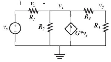
Let  $R_1 = 1 \text{ k}\Omega$ ,  $R_2 = 2 \text{ k}\Omega$ ,  $R_3 = 3 \text{ k}\Omega$ ,  $R_4 = 4 \text{ k}\Omega$ , G = 5 mS,  $v_s = 2.5 \text{ V}$ .
