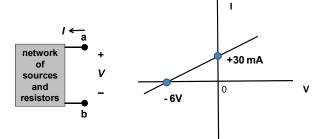
(a) (6 points) Calculate values of the Norton Current  $I_N$  and the Norton Equivalent resistance  $R_N$ .
