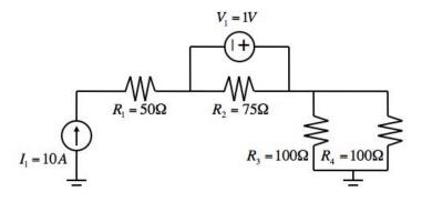
For the circuit above, mark all currents you will use to analyse the circuit on the figure. Determine the current values flowing through  $R_2$ ,  $R_3$  and  $R_4$
