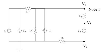
a) (7 pts) Does the current source  $I_{S1}$  have impact on voltages  $V_1$  and  $V_2$ ? Justify your answer. (Hint: You do not need to solve the rest of the problem to do this part!!)
