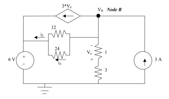
a) (4 points) Write  $V_a$  in terms of  $V_B$  (the voltage at node B). VA=-1/4VB (by Voltage Divider Equation)
