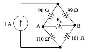
Current in each path is equal at 0.5 A. Vab = 0.5 (110-101)=4.5V
