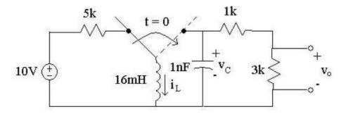
Assume the switch has been to the left for a long time before switching to the right at t = 0.
