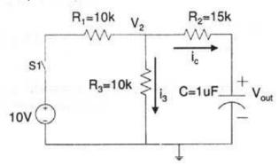
(a) (12 pts) Construct the differential equation of  $V_{out}$  in terms of all the given quantities. Hint: you may solve this use Mesh of Nodal analysis, or even simpler, Thevnin equivalent circuit. Write all your steps.
