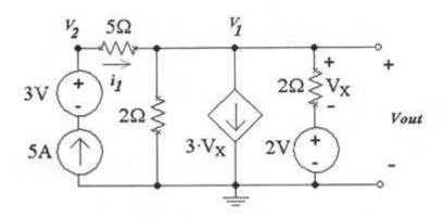
(b) (5pts) Use KVL, write down the equation of  $V_{x}$  in terms of  $V_{1}\,\mbox{and/or}\,V_{2}$
