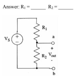
[5] b. Find the Thevenin equivalent circuit at terminals a, b for the circuit of Part a. Make your method clear. Give both the values and units in your answer.
