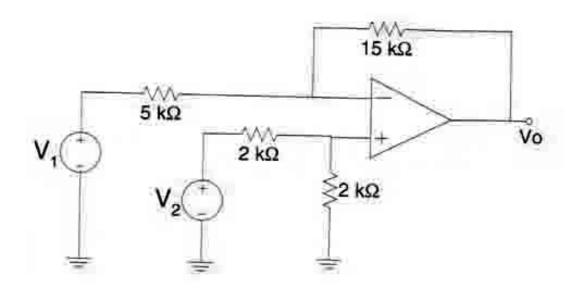
Design an operational amplifier circuit that has an output voltage  $V_0 = 3 V_2 - 5 V_1$ . The input voltage sources  $V_1$  and  $V_2$  cannot be detached from ground, and each have their negative terminals at ground. Assume that your amplifier is operating linearly.
