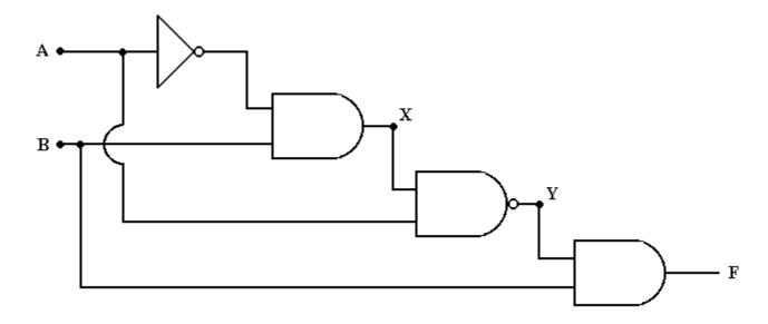
(a) Given the input waveforms for A and B versus time shown, make a neat sketch of the logic response versus time for the nodes X, Y, and F. (Assume that the values of A and B given at t=0 were the same for a long time before 0.) Important: Make your timing sketch on the area provided below. Do this independently of part b. Hint: For your own use, you may want to sketch the invert of A on top of the graph for A.
