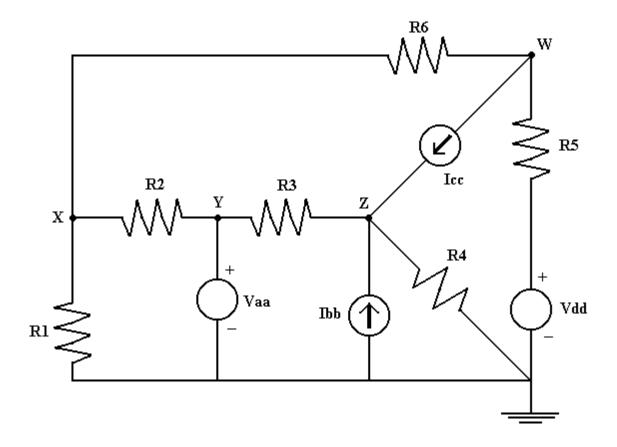
(a) In this problem you are to use nodal analysis to find a set of equations enabling you to find the values of VX, VY, VZ, and VW. First, identify which of the four are really unknown node voltages and secondly, write sufficient equations to find the four values. Hint: If, for example, two of the voltages are known, you first write these two values (known node voltages), then you would need twp nodal equations for the two unknowns.
