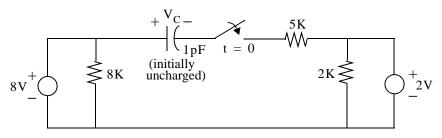
For the circuit above, the capacitor is initially uncharged. The switch closes at t = 0.
