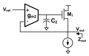
a) (6 pts) As a function of  $g_{m1}$ ,  $g_{m2}$ , and  $C_2$ , what is the s-domain output impedance  $Z_{out}(s)$  of the circuit shown above?
