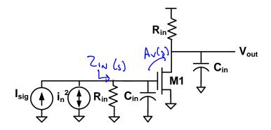
In this problem we will be examining the circuit shown above, where  $I_{sig}$  is a sinusoidal input current with an amplitude of  $A_I$  and angular frequency  $\omega$ , and  $i_n^2$  is a white noise current source with a power spectral density of  $4kT/R_n$ .
