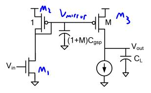
b) (5 pts) Now let's look at the stability of this amplifier under feedback using the model shown above (ignore the  $r_o$ 's and all capacitors except the ones shown in the model). If the amplifier is placed into unity-gain feedback with a closed-loop bandwidth of  $\omega_{gbw}$ , what is the maximum M that will provide at least 45° of phase margin? You should provide your answer in terms of  $\omega_{gbw}$  and the  $\omega_T$  of the PMOS transistors.
