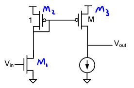
a) (4 pts) Assuming that the V\* of the NMOS and PMOS transistors are  $V_n^*$  and  $V_p^*$  respectively and ignoring the  $r_0$  of all of the transistors, what is the nf of the amplifier shown above? In other words, relative to the noise current from the input transistor, what is the noise current density that flows into the amplifier's output? You should provide your answer in terms of  $V_n^*$ ,  $V_p^*$ , and M.
