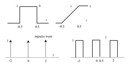
Figure 5: Impulse reponse, step response, impulsetrain and response for Problem8
