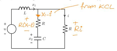
a) (5 points) Write an expression for the current *i* indicated on the circuit diagram in terms of  $x_1$  (the inductor current) and  $x_2$  (the capacitor voltage). Your answer should **not** involve any derivatives.
