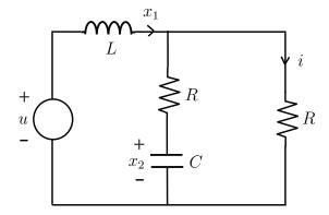
a) (5 points) Write an expression for the current i indicated on the circuit diagram in terms of  $x_1$  (the inductor current) and  $x_2$  (the capacitor voltage). Your answer should <u>not</u> involve any derivatives.
