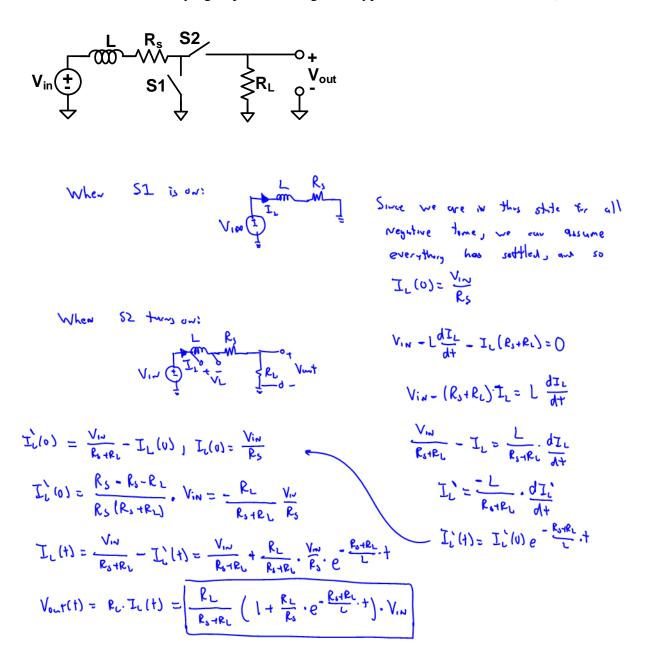
c) (4 pts) Assuming that after plugging in values for the various circuit components your answer to part b) was that  $V_{out}(t) = 1V + 2V * e^{(-t/500ns)}$ , how long after changing the state of the switches (at t=0) will it take for  $V_{out}(t)$  to reach 2V?
