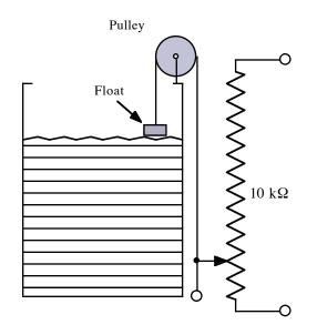
**4.1** (10 points) Design a circuit that produces a 10 V output when the tank is full and 0V when the tank is empty. The output must drive the recording circuit which acts as an approximate 10 k $\Omega$  load.
