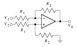
**2.2** (10 points) Using the equation derived in part 2.1, write an equation for the differential and common-mode gains as functions of the resistors  $R_1$  and  $R_2$ .
