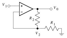
The op-amp has open loop gain A = k/f,  $k = 10^6$  Hz and the input impedances are infinite.
