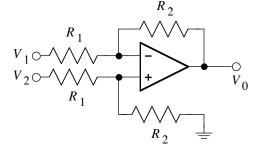
Infinite open-loop op-amp gain: virtual short rule:  $V_+ = V_-$
