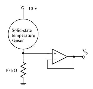
**4.3** (15 points) Derive the equation for the output voltage  $V_0$  in the circuit below as a function of the furnace temperature  $T_f$  and the room temperature  $T_r$ .
