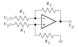
**2.2** (15 points) Using the equation derived in part 2.1, write an equation for the differential and common-mode gains as functions of the resistors  $R_1$  and  $R_2$ .
