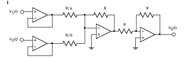
The first stage provides high input impedance, the second stage is a summing amplifier that also inverts the sum, and the final stage re-inverts the signal. The minimal solution requires five resistors and four op-amps.
