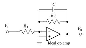
2d (5 points) For voltage gains of 10.00 at 0 Hz and 7.07 at 1 kHz, specify suitable values for  $R_1$ .  $R_2$ , and C.
