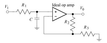
**2b** (5 points) For voltage gains of 10.00 at 0 Hz and 7.07 at 1 kHz, specify suitable values for  $R_1$ .  $R_2$ ,  $R_3$ , and C. (Hint: For RC = 0.159 ms,  $1/(2\pi RC) = 1$  kHz)
