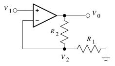
The op-amp has open loop gain A = k/f,  $k = 10^7$  Hz and the input impedances are infinite.
