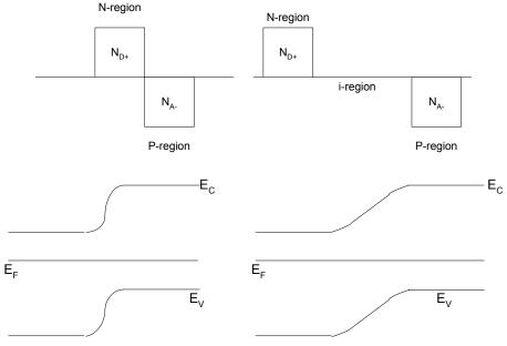
b) As you will see in your next class, PIN junctions are commonly used in photodetectors. Aside from this application, PIN diodes are also popular for use in high-speed circuits, since the typically show faster switching response than equivalent PN diodes. Why is this true? To justify your answer, derive an equation for the C-V characteristics of a PIN diode, and contrast it to a PN diode.
