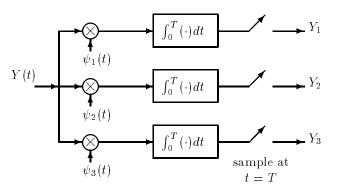
$\{Y_i = \int_0^T Y(t)\psi_i(t)dt\}|_{i=1}^3$  are sufficient statistics for optimal detection. Three sufficient statistics are needed because there are three basis signals for the signal set.
