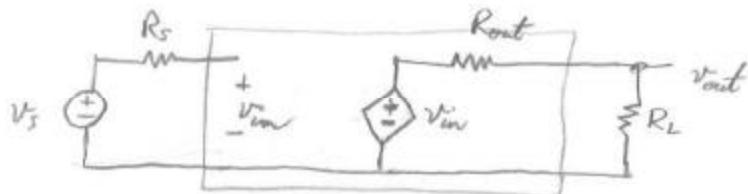
$$v_{out} / v_s = \frac{R_L}{R_{out} + R_L} = \frac{1000 \Omega}{454 \Omega + 1000 \Omega}$$
